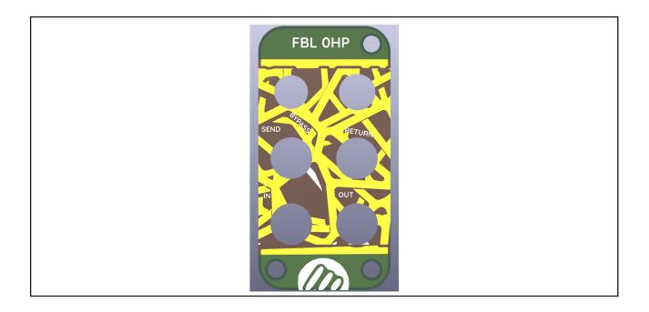
IN / SEND : connect to the output of another module/unit/fx OUT / RETURN: connect to the input of another module/unit/fx BYPASS: The bypass switch will stop the loop
